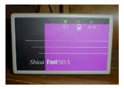
The FastPath 5 is an Ethernet (TCP/IP) to AppleTalk router/bridge. The software it uses is not only capable of basic routing of TCP/IP from Ethernet to AppleTalk cabling, it can also do quite a bit more.
