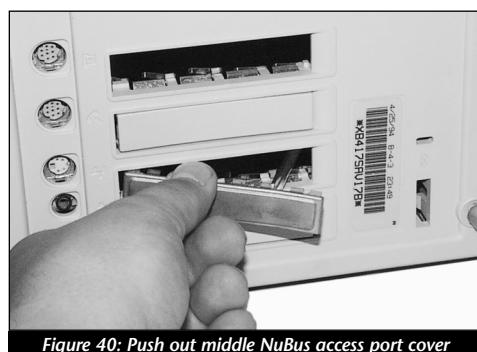
Figure 40: Push out middle NuBus access port cover
